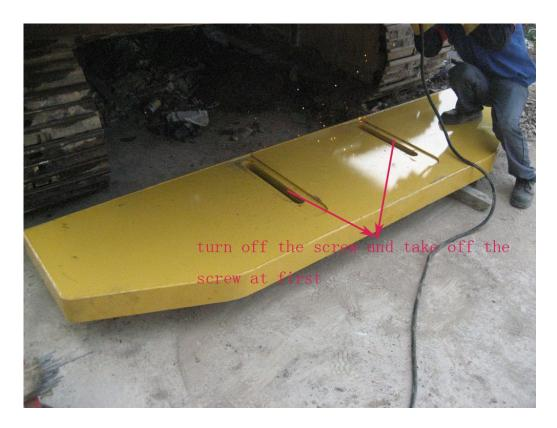
3. Weld the screw rod onto the excavator beam. See below photo .
