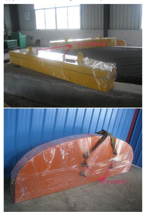
2. So you have to unscrew the counterweight (turn off screw) at first and put the unscrewed counterweight under the back of the excavator . See below photo
